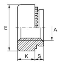
Female thread A = M3Height K = 2.0Max recess height = 1.0 Min distance to edge = 4.0Outer diameter E = 7.0 Plate thickness = 0.8 to 1.0
